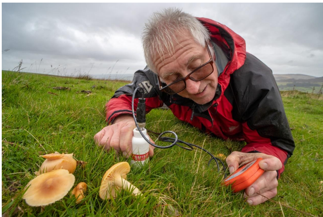
Measuring soil pH using a probe
