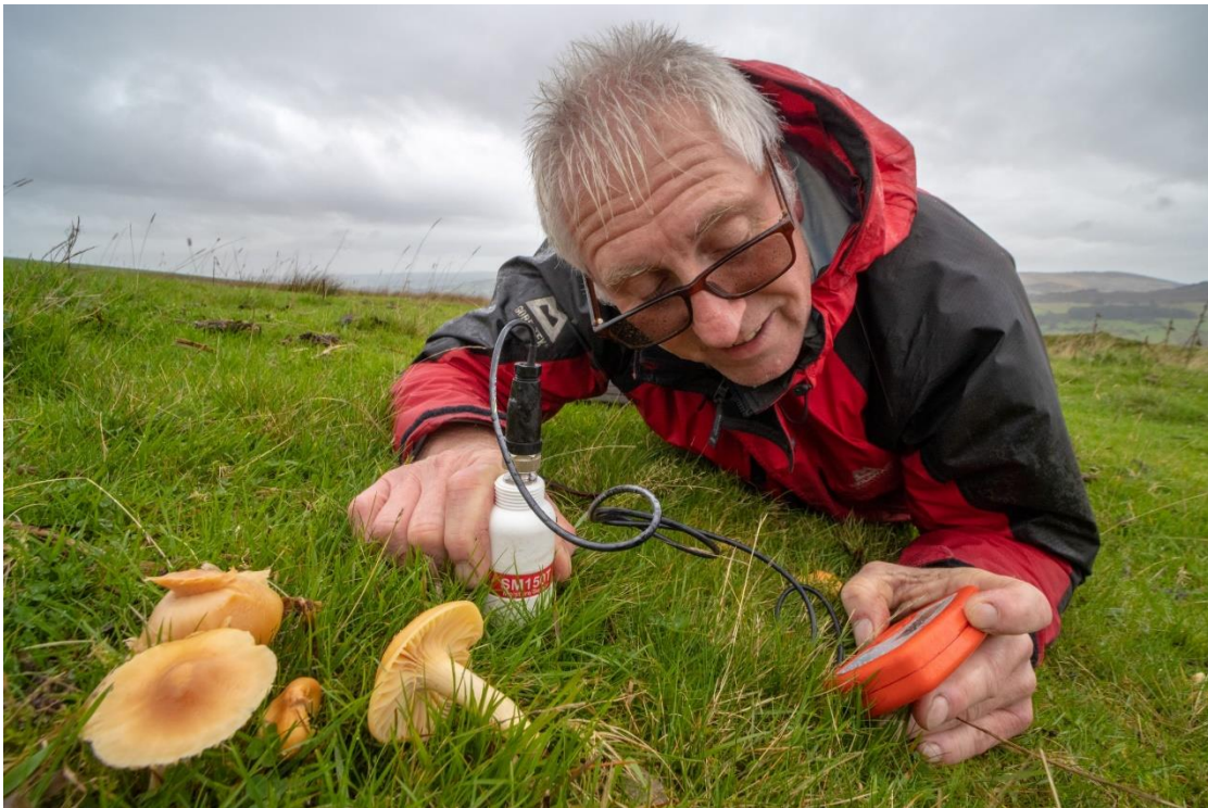
Measuring soil pH using a probe
