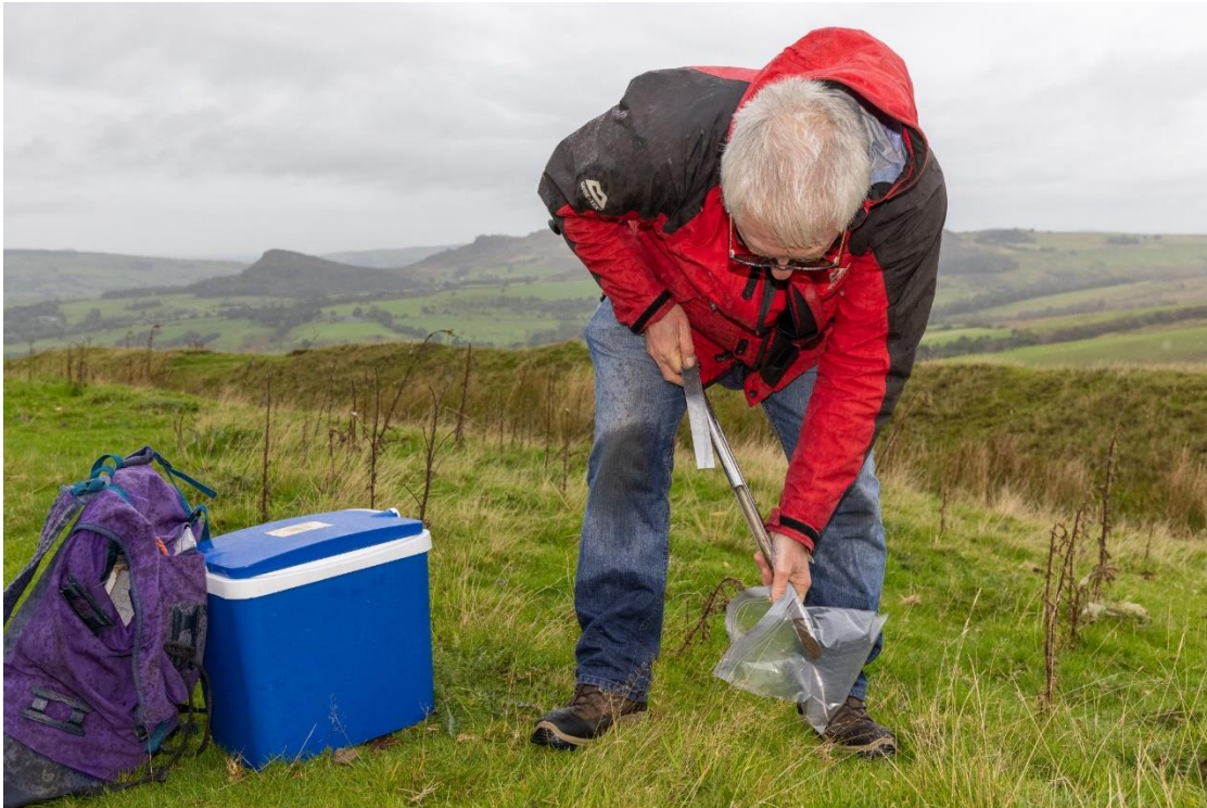
Collecting soil cores using an auger and transferring these to a plastic bag before chilling
